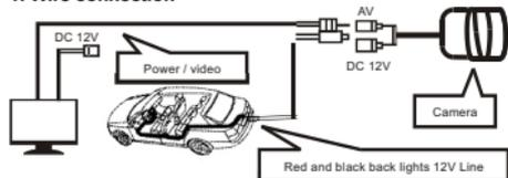
Complete all of the required connections in the way that make all the lines hidden in the car.
